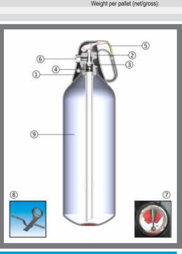
1) The handy compact valve is ergonomically designed to guarantee an easy use with one hand. The construction material of the cap ensures a perfect protection against corrosion. The safety button – PUSH 1 – and the operating button PUSH 2 – are clearly visible.
